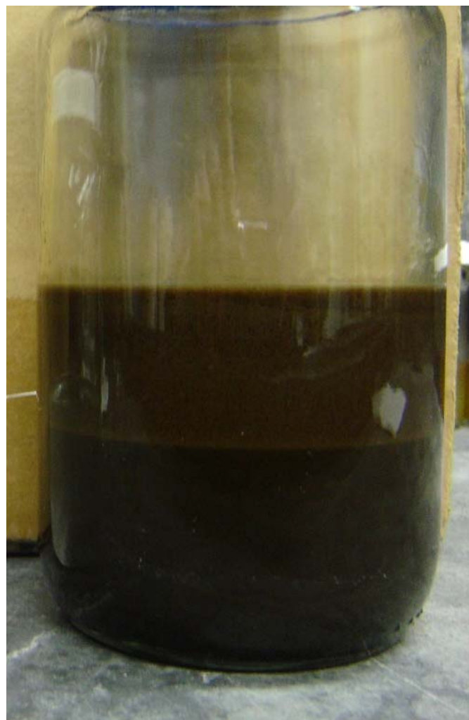
Concentrate from MVR 99.7 % Volume Reduction
