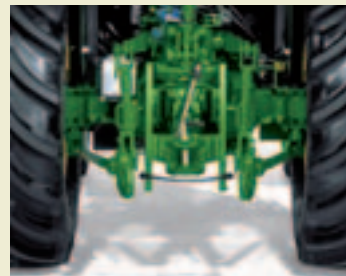
Seven position, height adjustable wagon hitch combined with drawbar makes hook-ups quick and easy.
