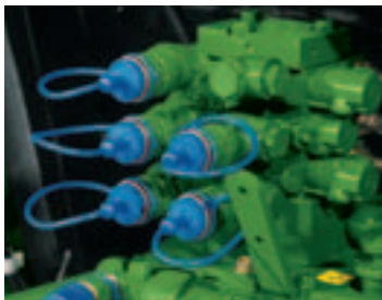
Rear SCVs deliver consistent flow for improved implement performance.
