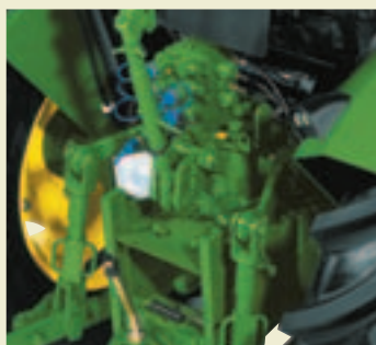
Checking oil levels is easy, too. The hydraulic and transmission oil fill and dipstick are located near the hitch in an easy to reach position.
