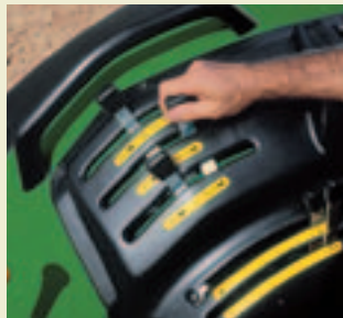
Range and gear lever, rockshaft and SCV controls are located on the operator's right. The PTO engagement and control of the ground drive PTO, are located on the left. All controls are positioned logically for easy reach.
