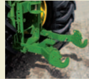
Optional quick couplers enable you to hook up implements quickly and easily from the operator's seat.
