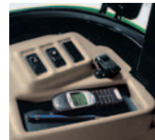
An optional 4WD and toggle switch with electro-hydraulic engagement lets you easily engage four wheel drive on-the-go when needed (available on all transmissions featuring Hi-Lo).
