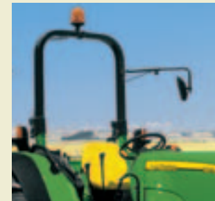
Choose between a two post, foldable ROPS (Roll Over Protection Structure) or a four post ROPS.
