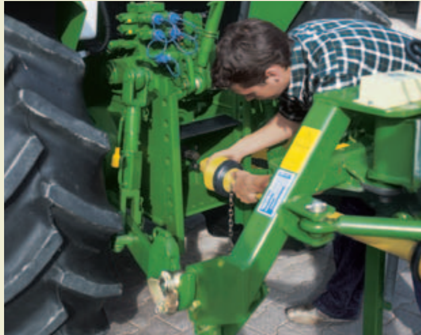
Optional quick couplers enable you to hook up implements quickly and easily from the operator's seat.
