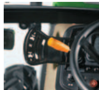
The Power Reverser gives you smooth and precise control for maximum productivity during loader operations.
