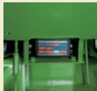
All open station models feature a covered fuse box to protect against water and dust.
