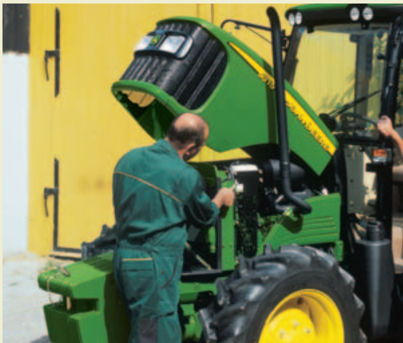
Servicing is easy. Lift the one-piece hood with integrated gas springs. Side panels remove for even greater access.
