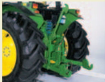
The heavy duty 3 point hitch lets you work with category II or I implements and lifts up to 26 kN throughout the whole lift range.
