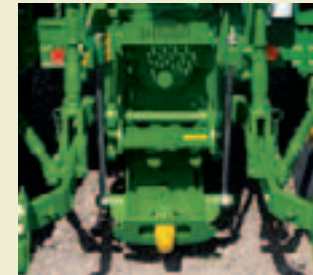
The optional pick-up hitch gives you an excellent view of the hook for easy coupling.
