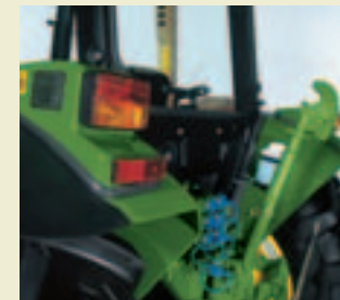
The electrical remote control (optional) for the 3 point hitch is mounted on the left fender.
