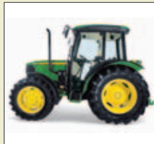
Select either a vertical or horizontal exhaust. The horizontal exhaust (shown above) improves visibility, making this choice ideal for front loader or row crop applications.
