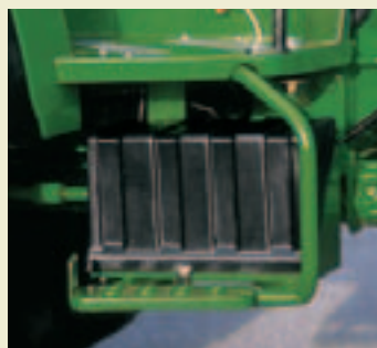
The relocated battery puts it within easy reach.
