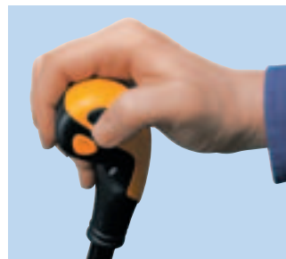
The 24F/12R Power Reverser transmission with a de-clutch button on the gearshift lever allows smooth and easy gear shifting without pressing the foot clutch pedal. 2 additional buttons let the operator control the electro-hydraulic Hi-Lo gear shifting.
