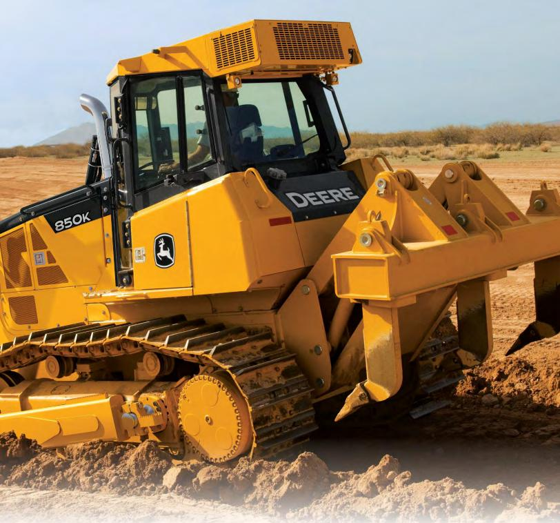
Flush-fit bottom guards and tight-fitting side shields help keep trash out. Hood and side-shield perforations function as a "first filter," further preventing entry of most debris. Anything that gets past the five-mm holes also passes through the cooler cores.
