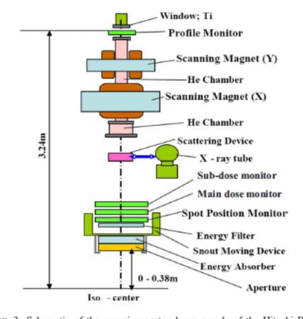
FIG. 3. Schematic of the scanning proton beam nozzle of the Hitachi Pro-Beat machine at PTC-H.
