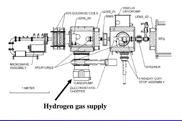
Microwave source based proton injector 20 keV injection energy
