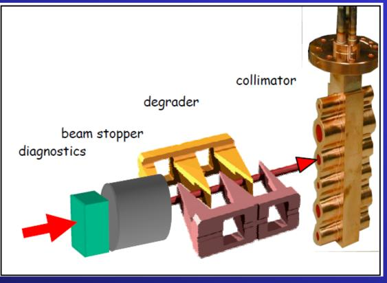
Energy modulation can be accomplished using a pair of opposed wedge degraders that operate on a 50ms time scale
