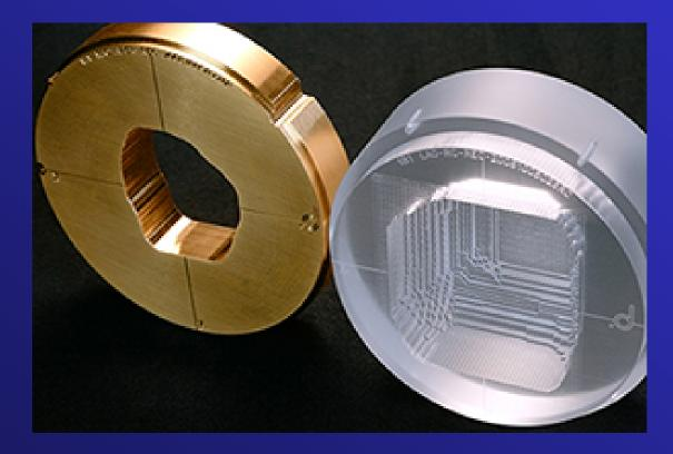
Brass collimator serves to collimate the incident beam inplane and cross-plane
