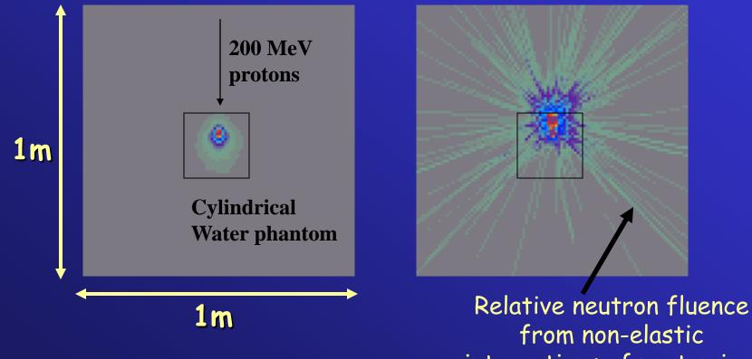
from non-elastic interactions of proton in a simulated brass collimator
