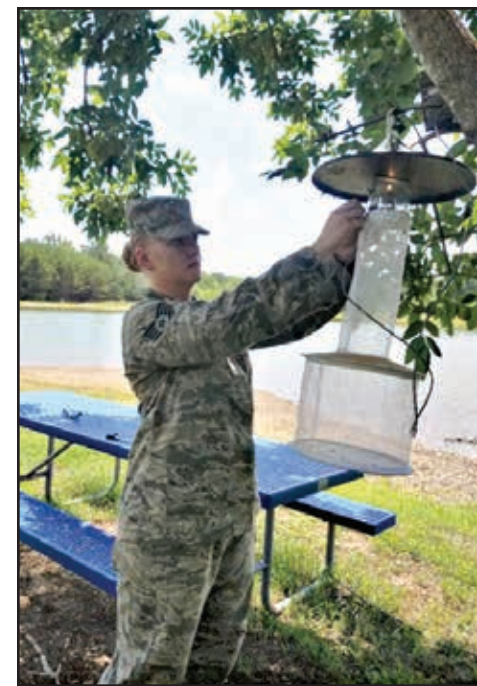
U.S. Air Force photo by Mr. Kenneth Durroh Staff Sgt. Viviana Chalfonte, 14th Medical Operations Squadrons NCO in charge of community health, hangs a New Jersey Light Trap for mosquito surveillance, June 27, 2018 on Columbus Air Force Base, Mississippi.
