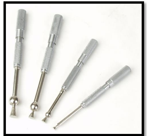
Small hole gages for measuring small tone holes and for setting trumpet valve slides parallel.
