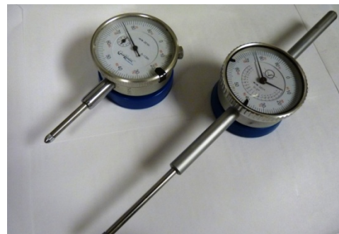
Flush mount magnetic base dial indicator (1" and 2" shown). Great for tracking tool bit travel.
