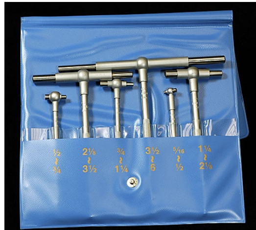
Telescoping gage set for measuring holes like valve casings
