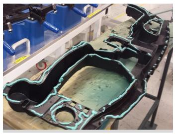
Figure 4. Lightweight glass-filled polyolefin bulk head moulding – being bonded with 3M<sup>™</sup> Scotch-Weld<sup>™</sup> Structural Plastic Adhesive DP8010NS Blue to an aluminum frame
