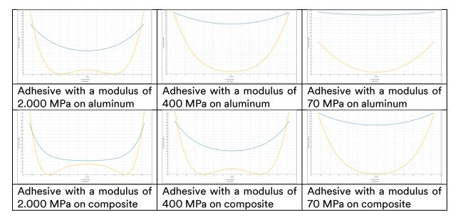
Figure 9: closed form calculations of stress within an adhesive joint as a function of modulus of the substrates and adhesive.
