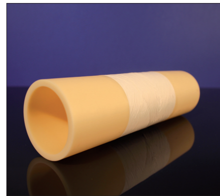
Fig. 15 Joined hybrid tube made of O-CMC and Al 2 O 3 liners for application temperatures up to 1200 °C
