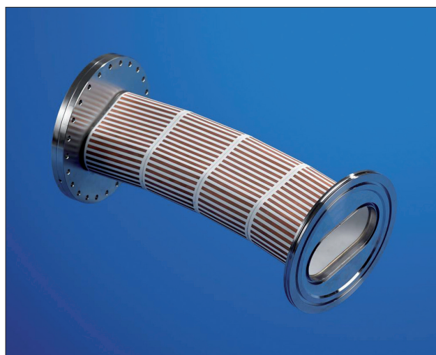
Fig. 1 Kicker tube of a particle accelerator, consisting of externally copper-plated \text{Al}_2\text{O}_3 with brazed metal flanges on the front edge [3]
