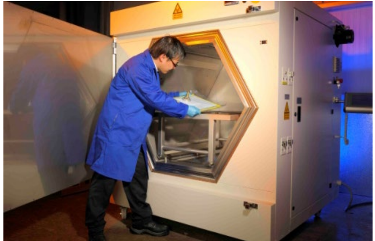
Figure 31: Commercial microwave oven designed for processing composites. Copyright © 2020 TWI Ltd reproduced with permission
