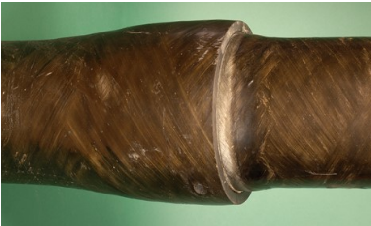
Figure 6: Mechanical interlock joint in a GFRP pipe. Copyright © 2020 TWI Ltd reproduced with permission
