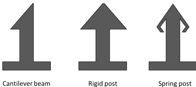
Figure 8: Three examples of locking features for mechanical attachment (Adapted from Messler, 1997 5 )
