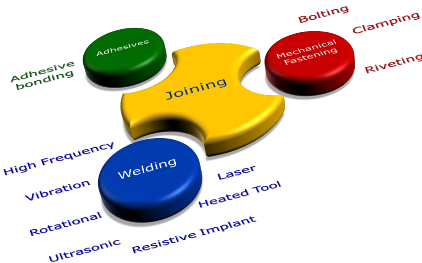
Figure 4: Summary of a selection of joining processes: bonding, welding and fastening
