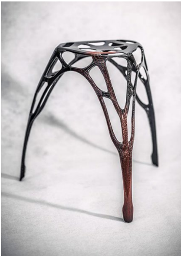
Figure 2: Leibniz Institute of Polymer Research (IPF, Dresden, Germany), the inventors of TFP, produced the preform for this stool using the process. Photo: IPF
