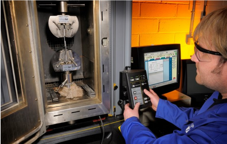
Figure 40: Single lap shear testing of an adhesively bonded joint. Copyright © 2020 TWI Ltd reproduced with permission
