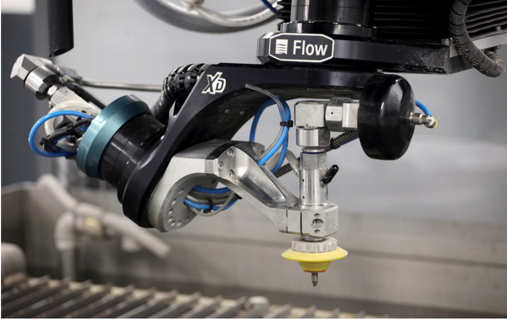
Figure 11: Water-jet cutter head. Photo: National Composites Centre
