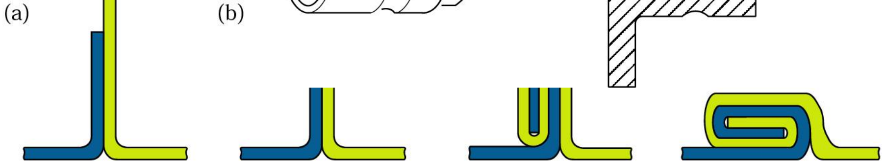
Figure 30.14 Stages in forming a double-lock seam.
