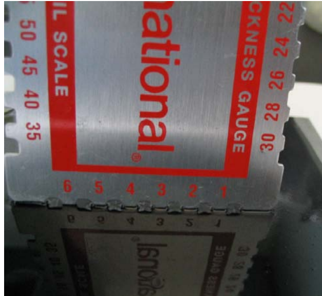
Figure 4. WFT Gauge Positioned in Wet Paint Film.
