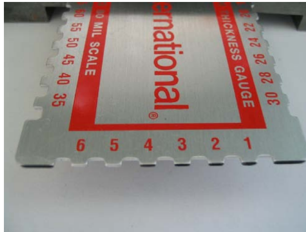
Figure 5. WFT Gauge Showing a Reading of 4-5 Mil.
