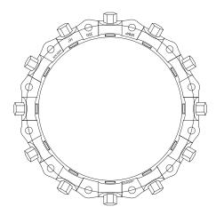
Mechanical Joint, Wedge Action Restraint for use on all classes of Ductile Iron Pipe
