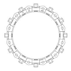
The Oversized Mechanical Joint Wedge Action Restraint has the same features as the Series 3000 except the bore ID has been increased to accommodate Class A, B, C & D pit cast pipe.
