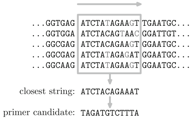
Fig. 7 Illustration to show how DNA primer design can be achieved by solving CLOSEST STRING instances on length- \ell windows of aligned DNA sequences. The primer candidate is not the computed consensus string but its nucleotide-wise complement
