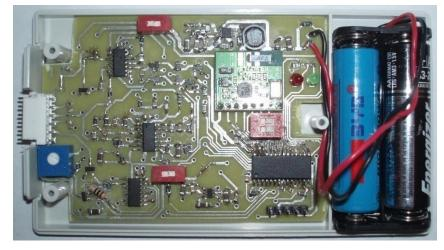
Two rugged, final sensor/transmitter prototypes were made for final product verification.
