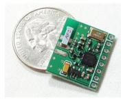
Figure 41: Nordic nrf24L01 transceiver chip; as used in this design, mounted on a breakout board
