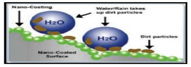
Fig. 3Nanocoatedself cleaning textile
