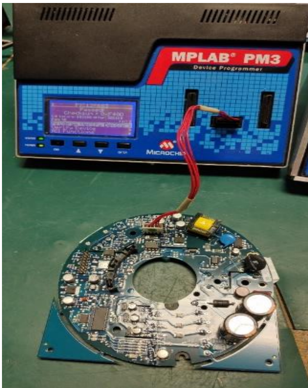
Figure 7 Parameter programming in a PCI Source: company case study
