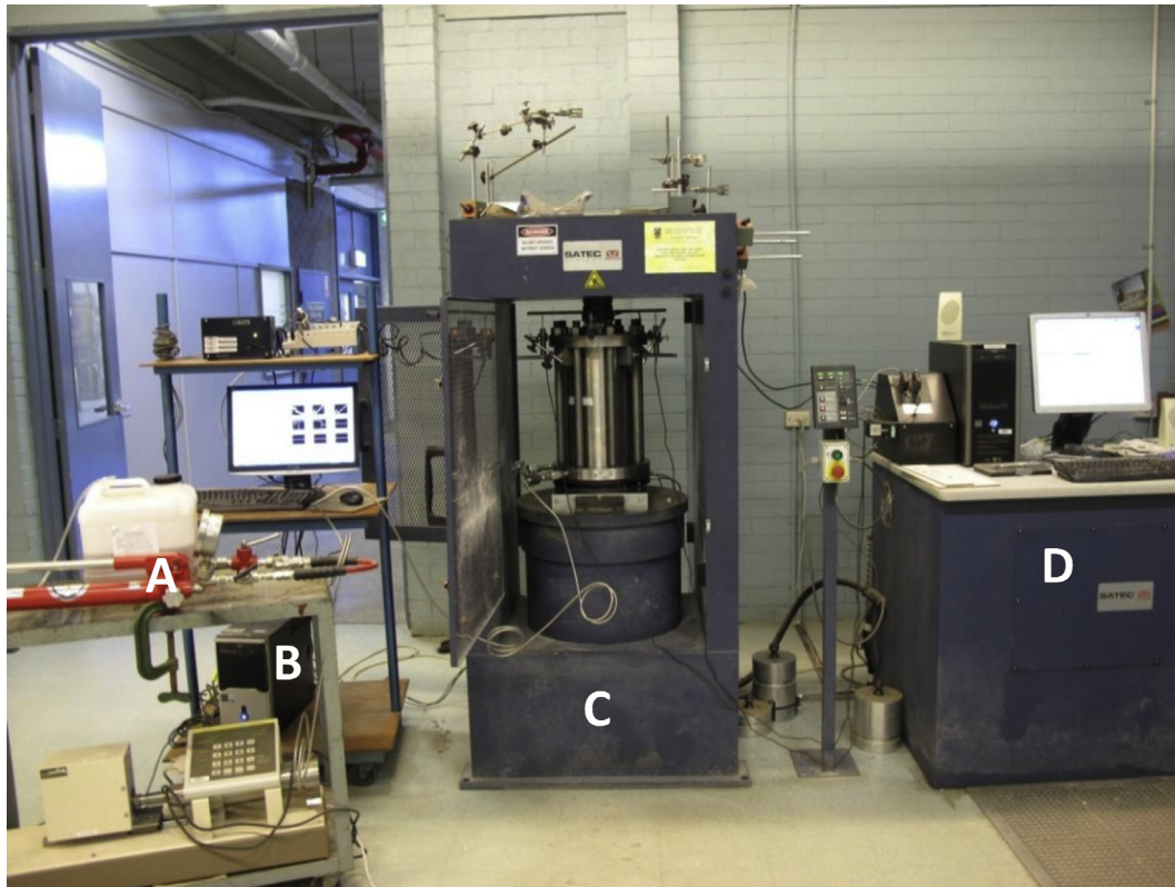
Fig. A1. Elements of the triaxial system: A- Hydraulic pump to provide and continuously control the confining pressure ( \pm 0.01 MPa), B- Computer system for data acquisition, C- Loading frame and D- The loading frame control system.
