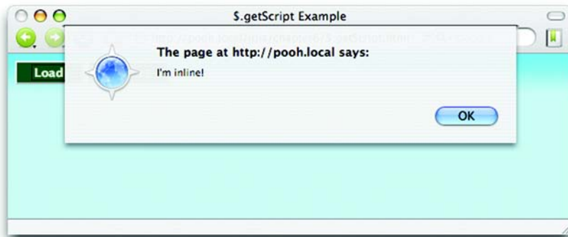
Figure 6.6 The dynamic loading and evaluation of the script file results in the inline alert statement being executed.
