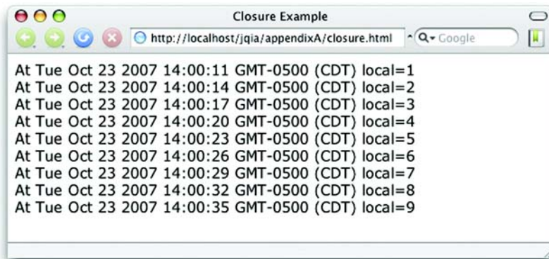
Figure A.5 Closures allow callbacks to access their environment even if that environment has gone out of scope.
