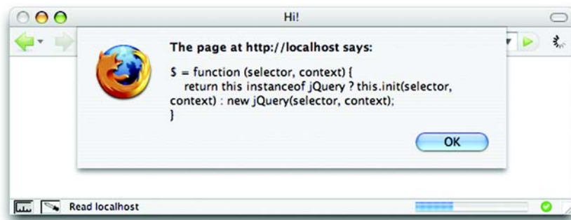
Figure 6.4 The alert now displays the jQuery version of $ because its definition has been enforced within the function.
