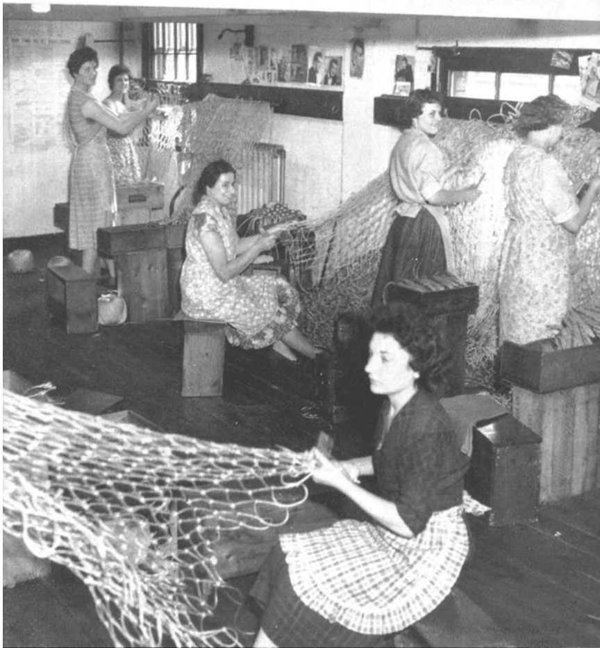
Braiding Nets Trawls are made up of several large pieces of net. The wings, belly and cod-end must be shaped so they fit together and the pieces are "increased" or "decreased" rather like a piece of hand knitting. So far the machines used to make nets haven't been able to do this. Fishermen prefer trawls made by hand. The picture shows a braiding room in Grimsby.
