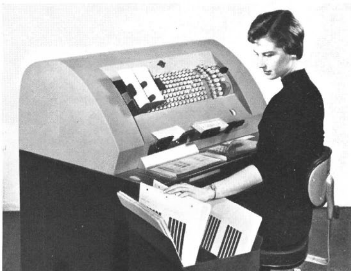
Book-keeper The National Post-tronic, a large book-keeping machine used in many American banks.
