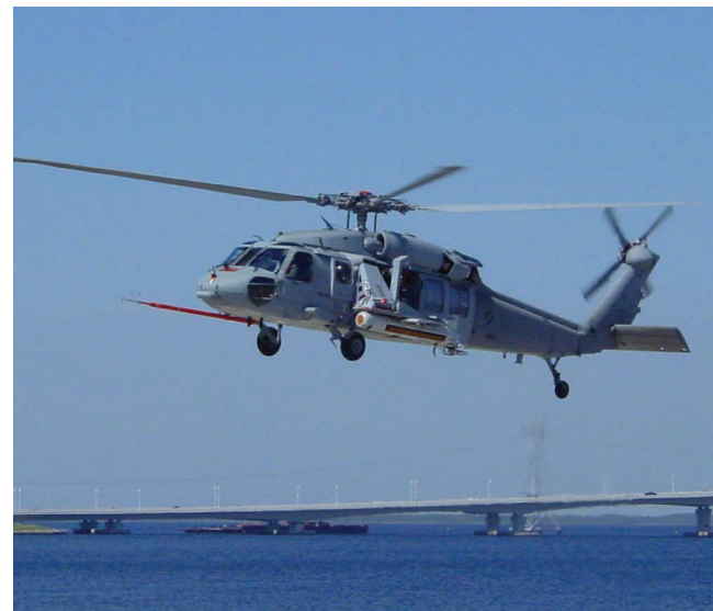
CSTRS was developed to enable the MH-60S helicopter to deploy mine countermeasure sensors in shallow water missions, providing an extra measure of safety for crew and ships.
