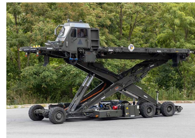
CTC developed a diesel-battery hybrid powertrain for the U.S. Air Force's Halvorsen 25K Loader, which is used to load and unload cargo from Air Force transport aircraft. CTC's solution improves agility, energy efficiency, and airman safety, while reducing greenhouse gas emissions.
