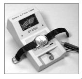
Besides checking batteries, this improved tester will also allow you to check the step-motor & coil.
