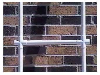
For this cage design, you need to push each PVC joint as tight as it'll go. The trick to that is to use your body weight to push the connectors onto the PVC.
