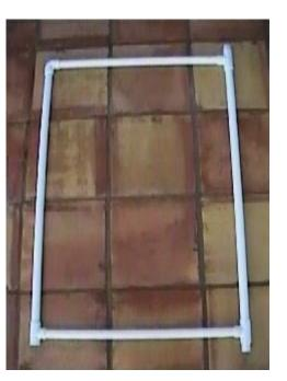
One more thing: there's a small gap that needs to be filled between the top and bottom sections of the door on the left side... so cut a [L] pole and connect the door sections together.
