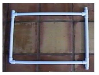
On the left side, put a 25 1/4" [D] pole, then a T connector facing out (to the left - see where it attaches to the frame),
