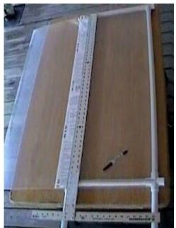
To cut the Lucite, I prefer an orbital jig saw with very sharp blades although people tell me that scoring both sides deeply and snapping gives a nice clean edge.
