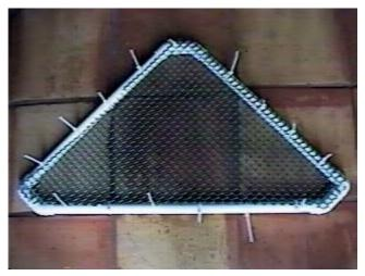
Using 3/4 pipe insulation, cover the frame.
