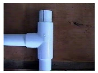
You can make the slots just by sawing into the plug once it's in the T.
