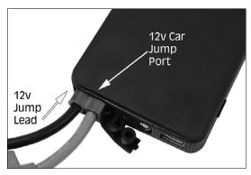
6. If the car fails to start on the first attempt, make sure all lead connections are correctly positioned. If, after 3 attempts to jump-start the car have failed, STOP, as this may damage the car and/or its electrical systems.
