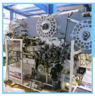
ACMA GD ACX-5E is a high speed stick gum wrapping machine and is complete with SF-breaker/feeder, with Allen Bradley Panelview 900 HMI. The wrap for the single piece is an inner wrap
