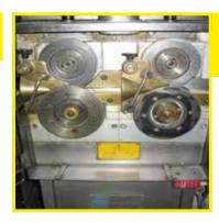
Euromec 8FL/1 single and 106FV/2 double stage rope sizers
