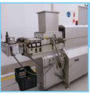
Bosch ball gum line that includes WEF1120 extruder, WAK0046 gum balling machine and WSC1200AE cooling tunnel
