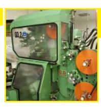
**GD 1001** high speed double twist wrapper for candy. Set on 24 x 15.5 x 10mm. Up to 1,000 p/m
