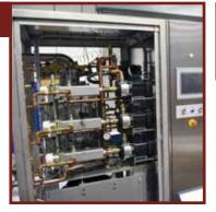
Chocolate drop-chip line includes Bindler GK8 drop depositor, and a Nielsen 600mm wide cooling tunnel, 12m long
