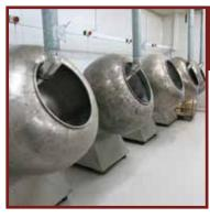
Various coating pans copper and stainless steel, used and rebuilt
