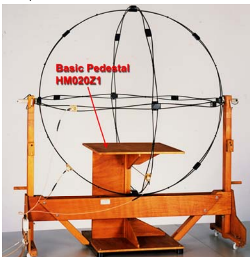
R&S®HM020 with a loop diameter of 2 m. Such LLAS can be used for EUT with a largest dimension of up to 1.6 m.
