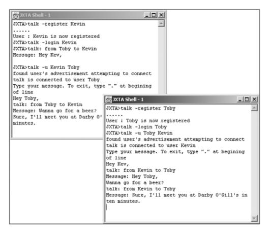
Figure 3.7. Using talk between two shell instances.
