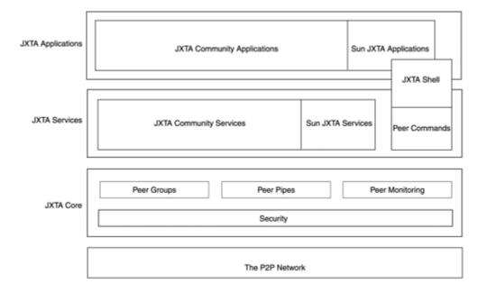
Figure 3.2. The JXTA three-layer architecture.
