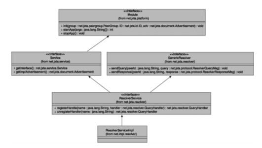
Figure 5.4. The Resolver service interfaces and classes.
