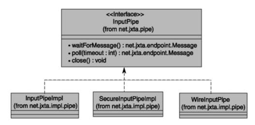
Figure 8.3. The pipe interfaces and classes.
