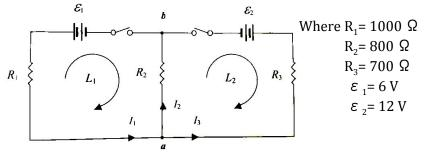
Then we measured the currents  $I_1, I_2$ , and  $I_3$  with an ammeter and calculated the currents using a system of equations utilizing Kirchhoff's *Junction* and *Loop* Rules, recording both values onto the data table.
