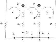
Where  $R_1 = 1000 \Omega$   $R_2 = 800 \Omega$   $R_3 = R_4 = 700 \Omega$   $\varepsilon_1 = 6 V$  $\varepsilon_2 = 12 V$
