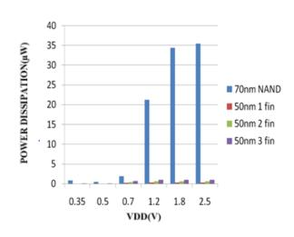
SUPPLY POWER DISSIPATION (µW) VOLTAGE VDD 70nm 50nm 50nm 50nm **(V**) NAND 1 Fin 2 Fin 3 Fin 0.35 0.851 0.024 0.044 0.065 0.5 0.447 0.033 0.06 0.087 0.7 1.897 0.245 0.457 0.664 1.2 21.227 0.315 0.628 0.941 34.332 0.314 0.629 0.943 1.8 0.941 2.5 35.376 0.315 0.63
