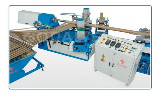
The Composite Can Making Plant is suitable to make Composite Cans for packaging of detergents, liquor bottles, automobile components, engineering goods, laminated cans for packaging of potato wafers, fruit drink, etc. These composite cans are eco-friendly as they are easily disposable and recyclable.
