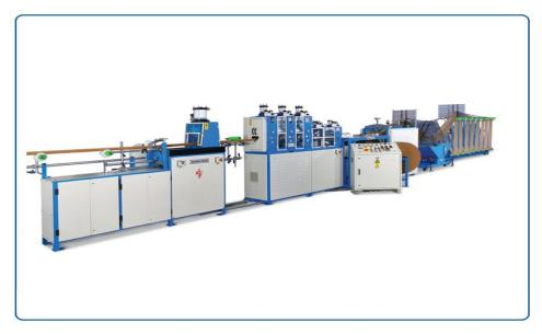
The Edge Protector Making Plant is made heavy duty to produce high strength paper edge protectors and 'U' Profile channels which are very ideal to prevent damages to edges of various palletized goods and circular goods like paper reels, steel coils etc.
