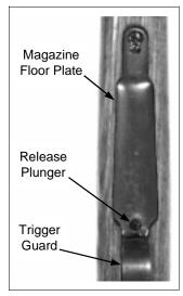
Fig 2 Magazine Floor Plate.
