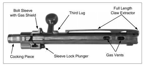
Fig 3. Bolt Assembly, Bottom View.
