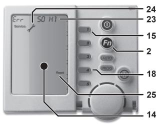
If the fault persists, use the ON/OFF button (1) to turn the Networker OFF, wait for 2 minutes before turning the Networker back ON. This may reset the heater and restore it back to normal operation.
