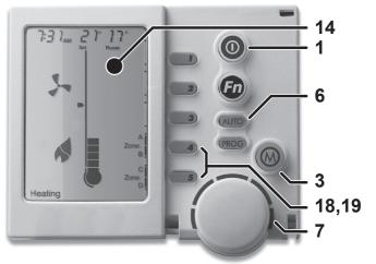
6. To turn the system OFF, press the On/Off button (1).
