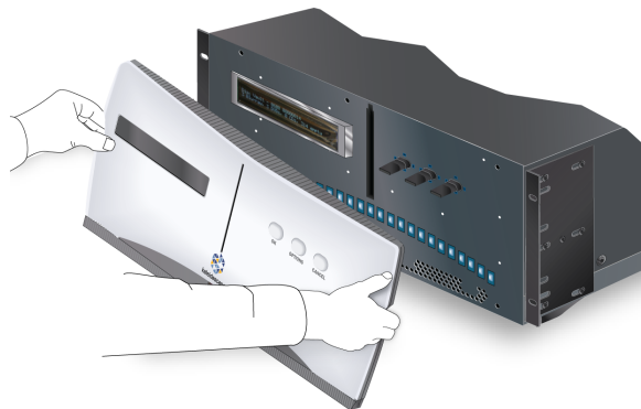
Figure 2 Removing the Front Panel
