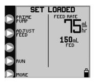
NOTE: If you have loaded the pump correctly and it continues to display "LOAD A SET", you may have a defective bag. See the troubleshooting section of this handout.
