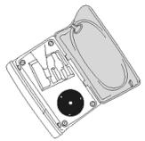
b. To load the tubing into the pump, grasp the finger tab on the light purple valve and slide the valve into the front channel of the pump. Make sure to push the valve all the way into the channel. Wrap the tubing around the rotor (wheel) and pull gently until you can slide the black ring into the back channel (DO NOT OVER-STRETCH THE TUBING).
