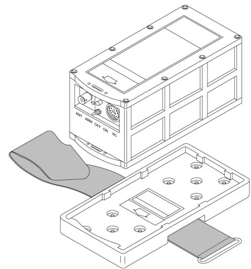
Figure 3: KANNAD 406 AF / AF-H / AF (6D) with mounting bracket
