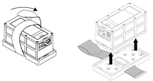
Figure 208: Removing the transmitter
