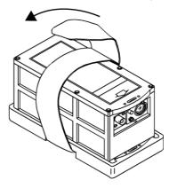
*Figure 203: Installing the transmitter on the bracket*
