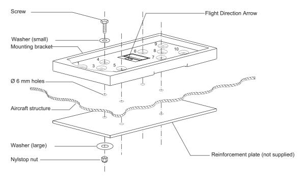
Figure 202: Bracket installation
