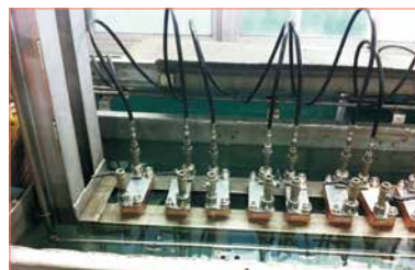
Pressure Leakage Test
