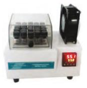
It is a closed reflux digestor used for digestion applications & can also be used for COD estimation with very small quantity of sample.
