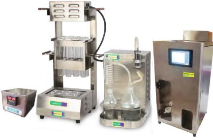
Spectralab Kjeldahl Nitrogen Analyzer KNA consist of a Digestion Unit, a Scrubber Unit & Steam Distillation Unit. Various models of digestors, scrubber & distillation unit are available. Our KNA leaflet describes this product in details which may be referred.
