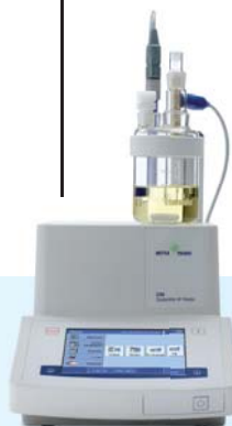
Water determination by Karl Fischer Titration
