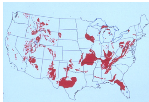
Figure 5. Karst Map of the United States – Karst areas highlighted in red. (Beck et al. 1996)
