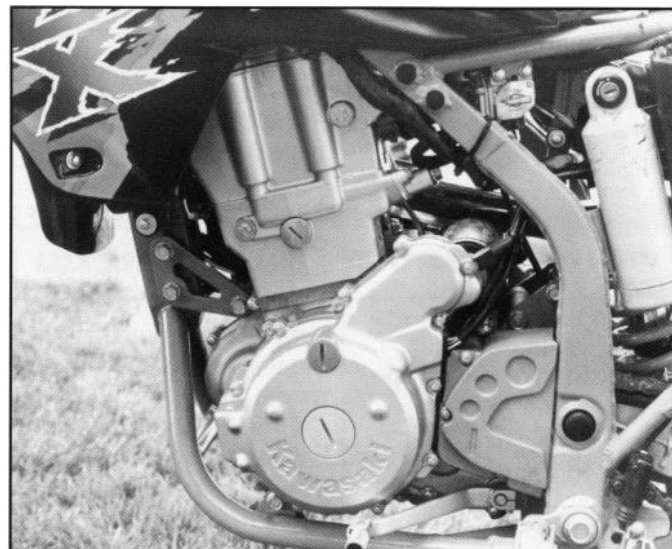
(LEFT) Front forks on the KLX650-A are inverted, feature 16-way compression damping adjustment and provide nearly 12" of front-wheel travel. (BELOW) 650-C engine has more low-end and mid-range torque and a conventional wet-lined cylinder. Larger side cover houses the electric starter.
