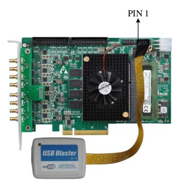
Figure 1: Komodo Frame Grabber board with USB-Blaster<sup>TM</sup> attached
