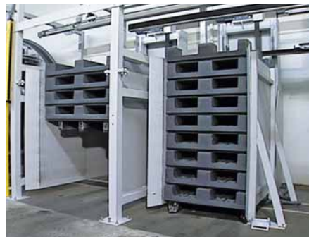
2: Fully automatic system pallet dispenser for the pile turner
