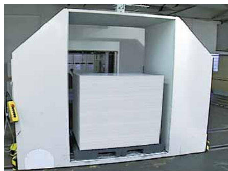
4: A remote-controlled trolley takes the pile from the roller track and brings it to the predetermined location. This location can be specified by way of an EAN code
