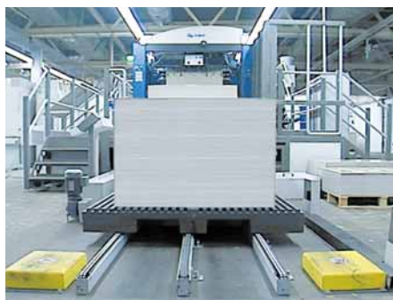
5: The pile is moved off the trolley and into the park position in front of the feeder
