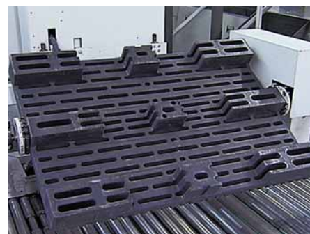
6: The empty pallets from the feeder are automatically turned, stacked and returned to the pallet dispenser at the pile turner
