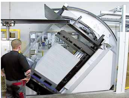
1: Pile turner: Replaces disposable pallets with non-stop system pallets
