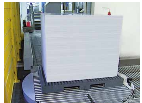
3: Turntable for routing of the pallets. Floor height differences can also be overcome with a lifting action
