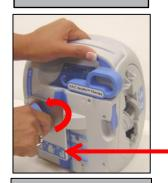
Turn the knob counterclockwise to unlock the hanger arm assembly.
