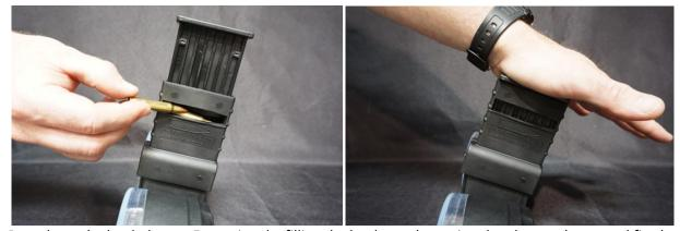
Rounds can be loaded up to 5 at a time by filling the loader and pressing the plunger downward firmly.
