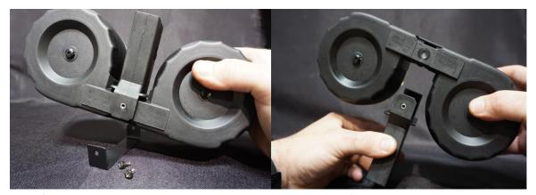
Set the floor plate and screws to the side and separate the tower from the magazine body. **NOTE** - Holding the magazine upside down will help to contain the followers inside the tower during disassembly
