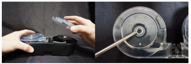
To reassemble, start by replacing the two rear covers and reinstalling the two screws that hold the covers to the drum.
