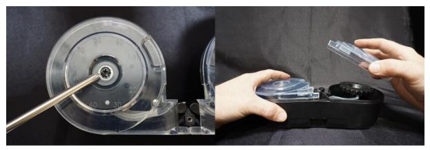
Remove the two screws in the center of the clear covers and set aside. The rear covers will then separate from the body by prying the covers up and outward from the center of the magazine body. This separation may require considerable force. Prying with tools is NOT RECOMMENDED as damage to the covers may occur.
