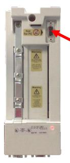
HSP-5 interface D-SUB 9-pole X4A: USB-serial-converter Part No. 00.58.060-0020
