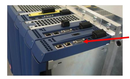
Connection drive units directly to serial D-SUB 9-pole protocol DIN 66019 II:
