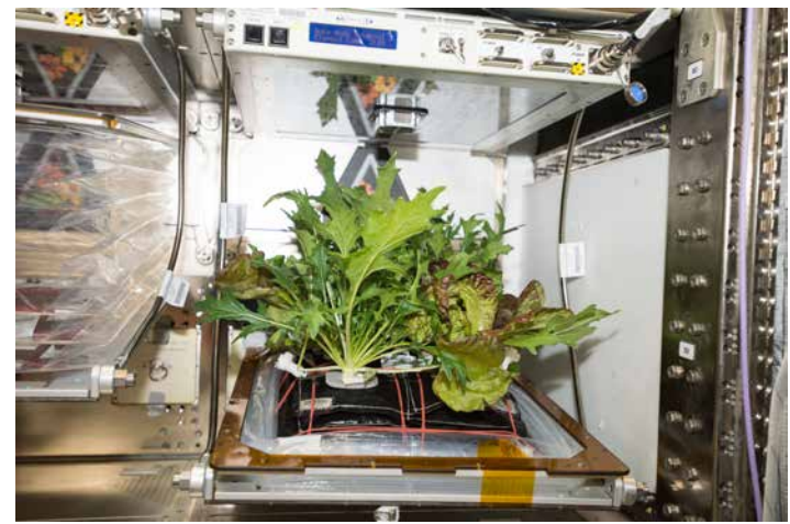
Three different varieties of plants growing in the Veggie plant growth chamber on the International Space Station were harvested Oct. 27, 2017. Photo credit: NASA/ISS
