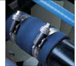
A standard item on Kenworth trucks, constant torque hose clamps go on tight and stay that way
