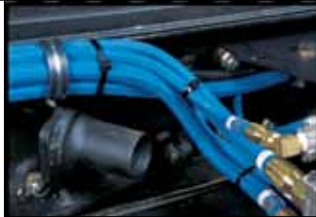
Kenworth offers wirebraided hose for its air brake systems – an extra that pays off in peace of mind when your application takes you miles from anywhere.
