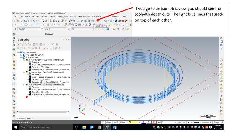
For the next procedure we want to verify the toolpath, basically we are going to virtually cut the piece on the computer. So we are going to look at the geometry and toolpaths in a 3D view so we can see what is going to happen better. Go to an isometric view if you did not already, zoom in\out, and center the work piece so it looks something like what is below.
