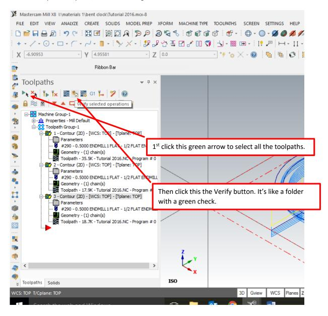
The MasterCAM Toolpath Simulator should open up in a new window. Like below.
