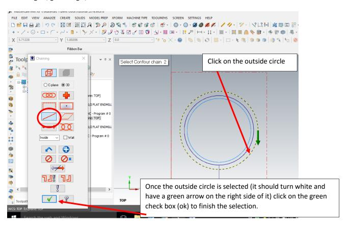
After you hit the OK button for selecting geometry for the toolpath, the 2D contour toolpath window pops up. This should have all the same settings we set for the first toolpath except for the depth. So you can check all the cut parameters and see if they are the same (they should be, if not just enter the same information for the last contour). Once you check the cut parameters, go to linking parameters and enter the **depth of -.375.**
