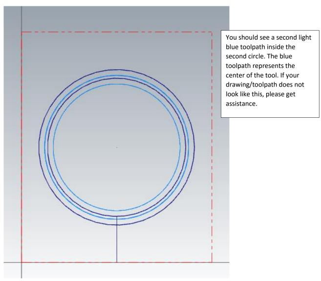
Now it's time for the plow for the dial and clock movement. This plow is represented by the small vertical line in the center of the clock front geometry. It is still a contour toolpath, so the procedure is similar. The only difference is the cutter compensation needs to be turned off, so the center of the cutter follows the line.
