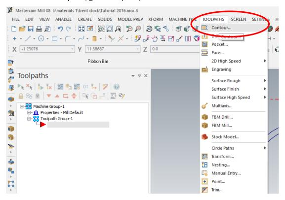
When the new NC dialog box comes up, type in a good file name such as Clock Front.
