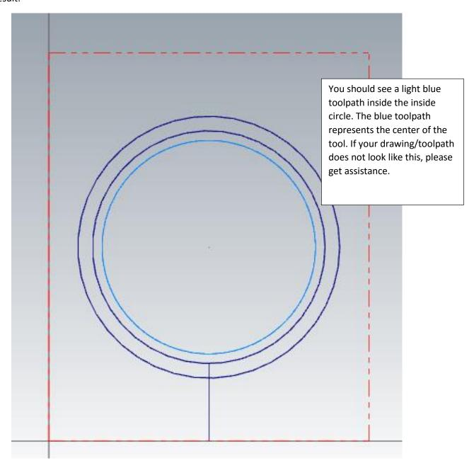
The second toolpath is similar to the first. It will be a contour with the same cut parameters and same tool, but we will not go all the way through the piece. This time we will make a rabbit, so the depth will be -3/8" or -.375.
