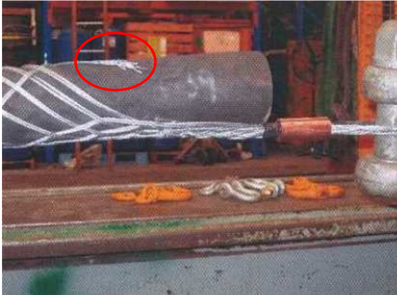
Entire strand on the metal whip-restraint failing, which can cause injury to personnel.
