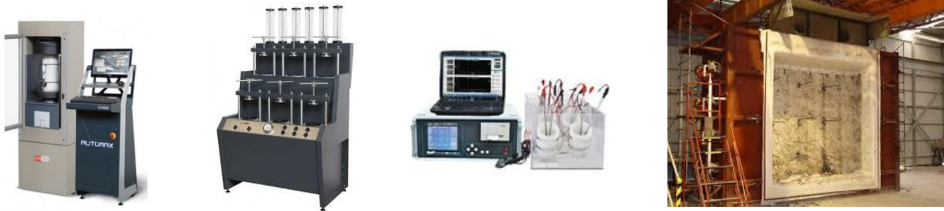
Setups for strength, permeability and fire resistance measurements
