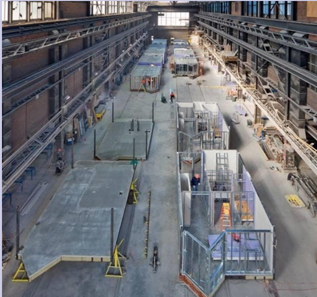
Manufacturing of fully furnished modular units in shop
