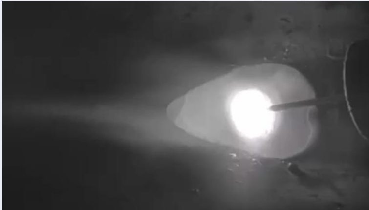
Lack of fusion ahead of arc due to low current
