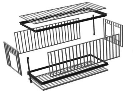
A steel modular unit
