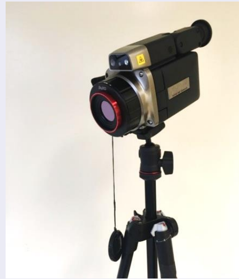
a) Infrared camera to record temperature history during welding
