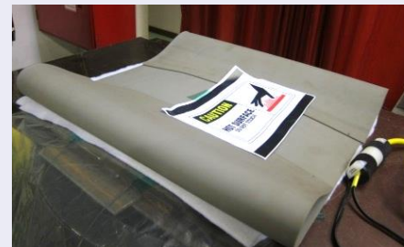
Electric blanket for pre-heating and post-heating
