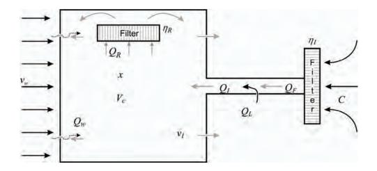
Figure E-1.—Schematic of basic cab filtration system.
