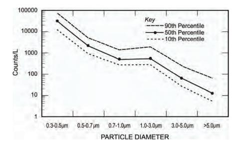
Figure 10.—Ambient air size classified particle count concentrations.
